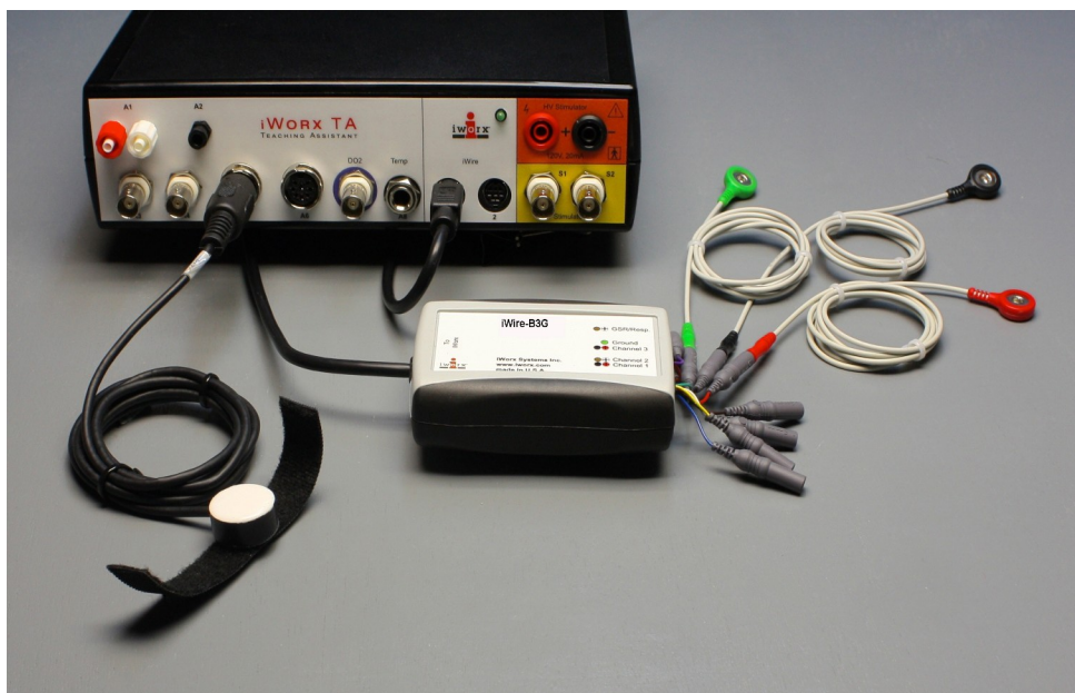
Figure HC-6-S2: A iWire-B3G ECG cable with 3 lead wires and the PT-104 pulse sensor connected to an IXTA. The Pulse Oximeter will be connected directly to the computer via USB.
